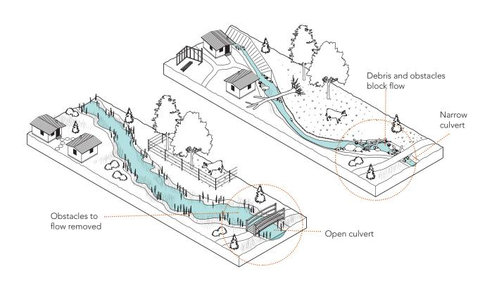
FIGURE 5.16 REMOVING BARRIERS TO FLOW
