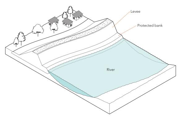
FIGURE 5.11 A LEVEE BETWEEN A WATER BODY AND DEVELOPED AREA
