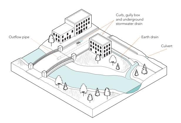
FIGURE 5.13 ENGINEERED DRAINAGE SYSTEMS
