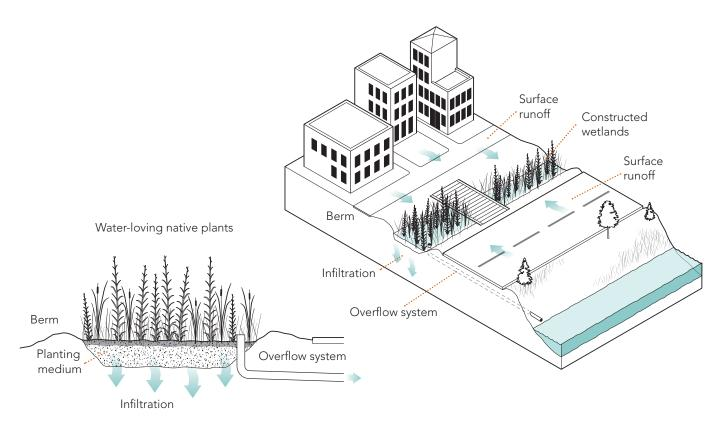
FIGURE 5.5 A TYPICAL CONSTRUCTED WETLAND DESIGN
