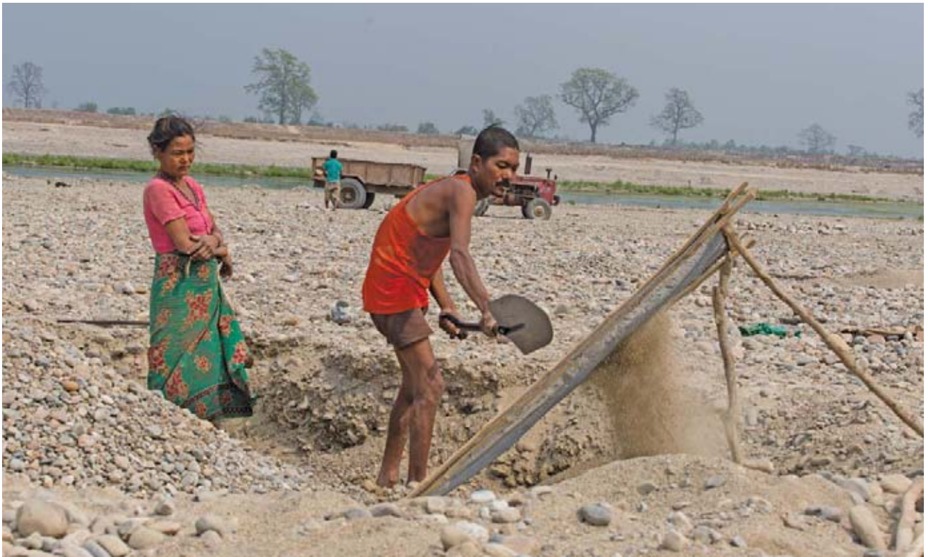
Extraction of sand, gravel and stone from rivers can destabilize the substrate and result in river bed material being scoured out during the next monsoon; the extra sediment is transported and deposited downstream where it can worsen flooding and river cutting. © WWF Nepal, Hariyo Ban Program/Nabin Baral
