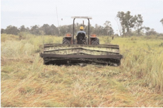
Photo 1: Rolling' the alang-lalang is the first step in the conversion process. After the roller has pressed ther alang-alang flat, chemical control using glyphosate is much easier and cost effective. The roller was manufactured by a local workshop.
