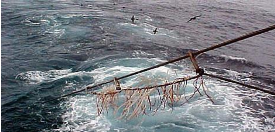
The contraption keeps seabirds away from the warp line of a trawler.
