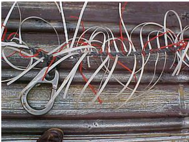
A close view of the rope, which looks like a bottlebrush.
